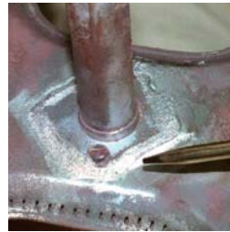
Pyro-Putty® 653 seals corroded burner manifold.
